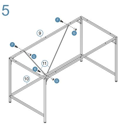
Attach frame [11] to frame [9] and [10] with 2 x bolt (F), bolt (E) and 3x nut (G). Tighten with a screwdriver.
