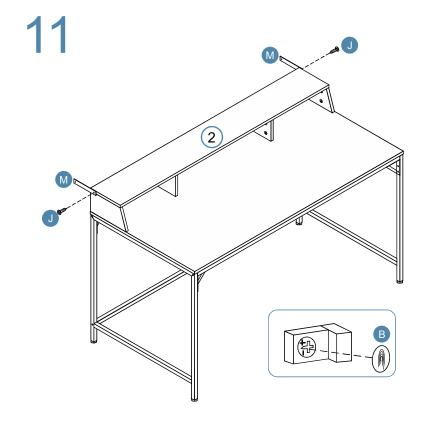
Attach safety strap (M) to panel [2] with 2 x screw(J). Then you can stick the PVC sticker on visible nut (A) to make the desk pretty.
