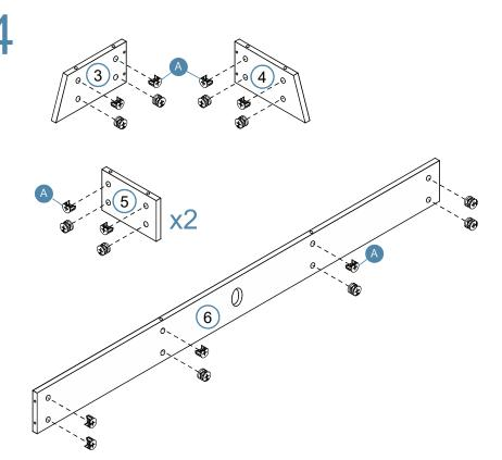
Insert 24 x nut (A) into panel [3], [4], [6] and 2x panel [5].
