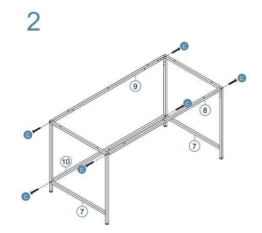
Attach frame [8], frame [9] and frame [10] to 2 x frame [7] with 6 x bolt (C). Tighten with a screwdriver.
