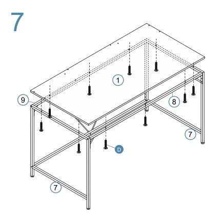
Attach panel [1] to metal frame with 10 x bolt (D). Tighten with a screwdriver.
