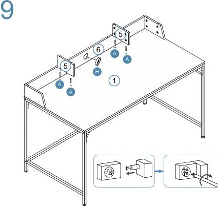
Attach 2 x panel [5] to panel [1] with 4 x bolt (A), and tighten with a screwdriver. Then insert organiser top (H) into panel [6].
