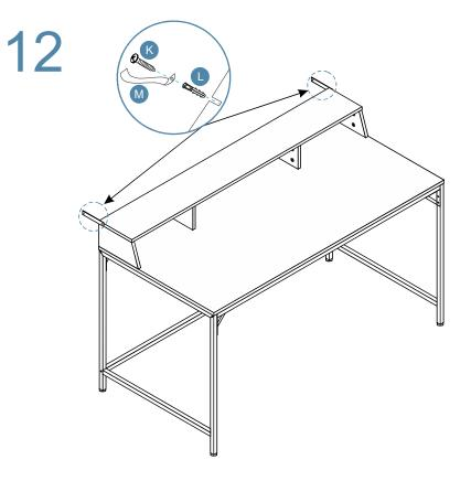
Move the unit to the desired location against a wall. Attach the other end of the 2 x safety straps (M) to the wall using 2 x wall plugs (L) and 2 x screws (K). Tighten with a screwdriver.
