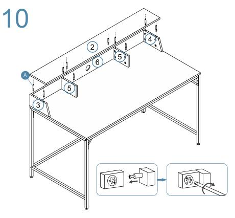
Attach panel [2] to panel [3], [4] and 2 x panel [5] with 10 x bolt (A). Tighten with a screwdriver.
