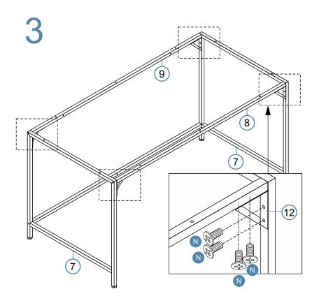
Attach the triangle frame [12] to metal frame [7], [8] and [9] with  $4 \ x \ bolt \ (N)$ .
